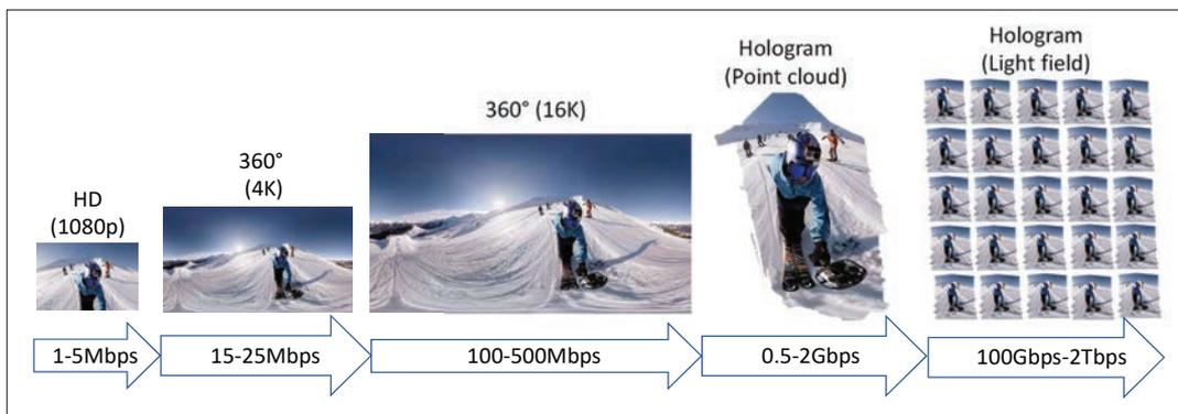
Figure 1. Bandwidth requirement evolution of video streaming services.
