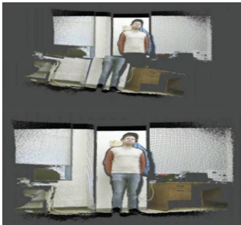
Figure 2. Images showing a misaligned (top) and a correctly aligned dataset [6].
