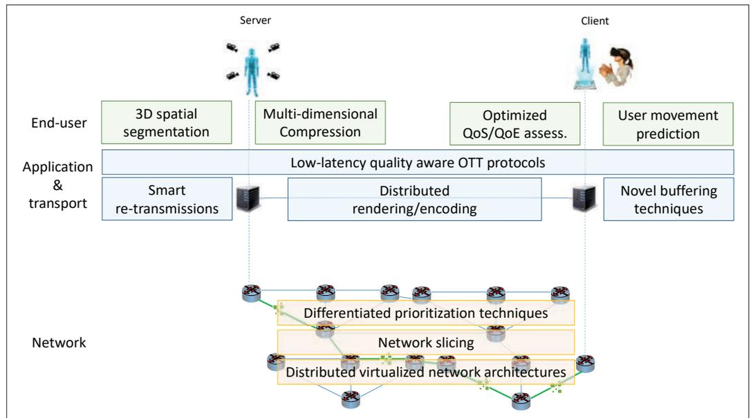
Figure 3. Challenges and solutions for a cross-layer optimization of infrastructure.
