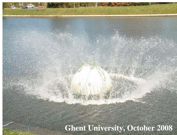
Figure 3 – Bottom slamming on large scale composite floaters at the Watersportbaan, Ghent.
