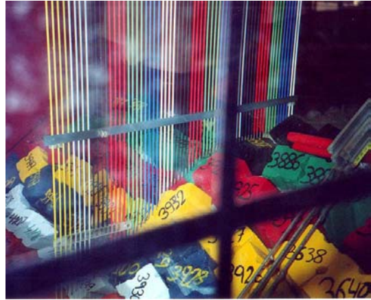
Fig 3. Photo of comb on a rubble mound breakwater slope, taken at the Universidad Politecnica de Valencia, Spain.
