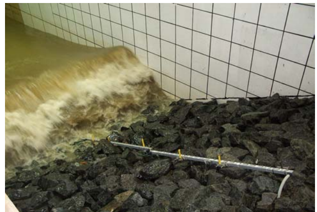
Fig. 4. Photo of the digital stepgauge at the Large Wave Flume in Hannover, Germany.
