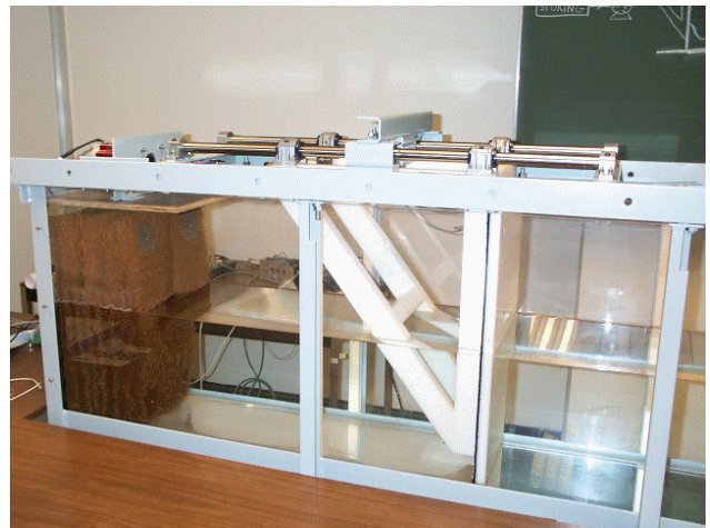
Fig. 2. Detailed view of piston type wave paddle.
