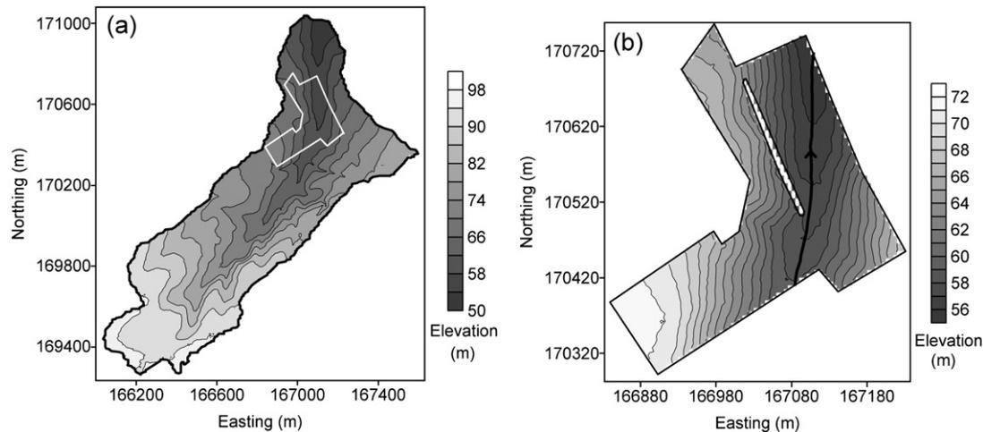
Fig. 1. (a) DEM of the smallest catchment enveloping the study field and (b) DEM of the study field indicated with the major drainage line; the topographic discontinuity is shown inside the study field.
